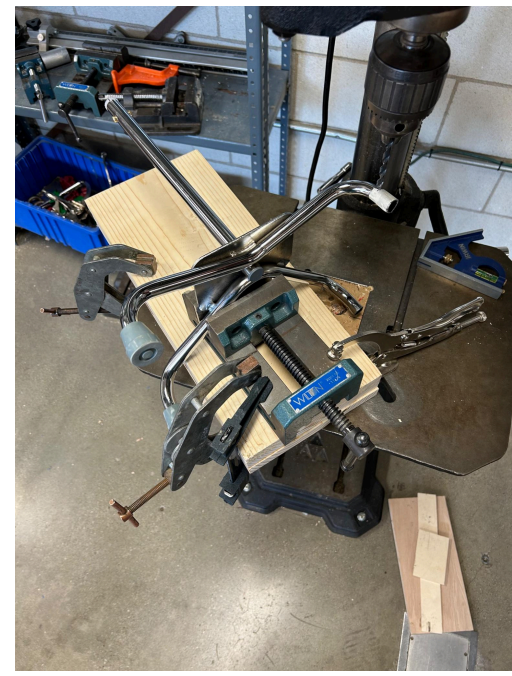
Fig. 4: Setup for drilling second axle hole
