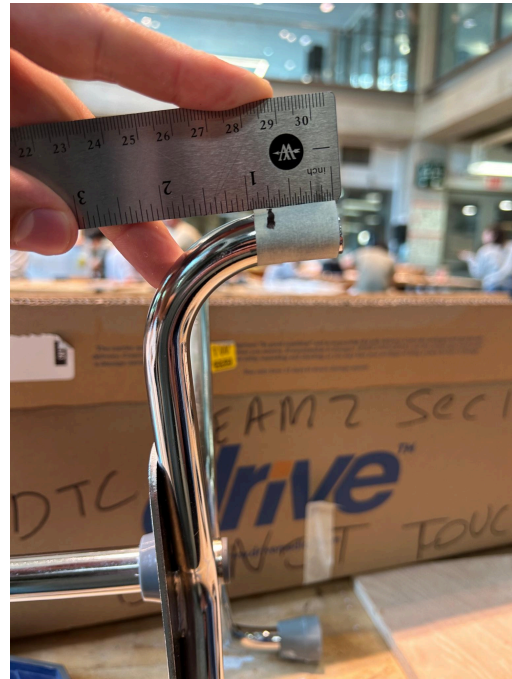
Fig. 2: Marking distance for axle holes
