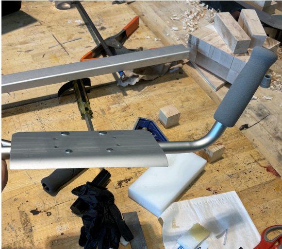
Figure 21: Inserted Grip Bar
