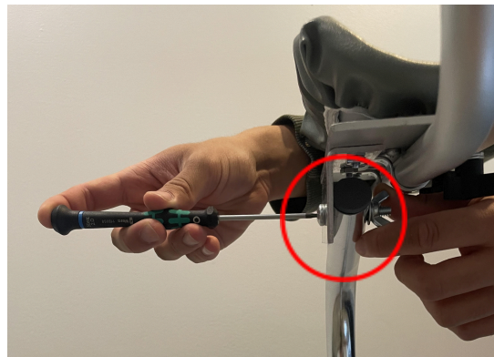
Fig. 6. Tightening Nut and Wing Nut
