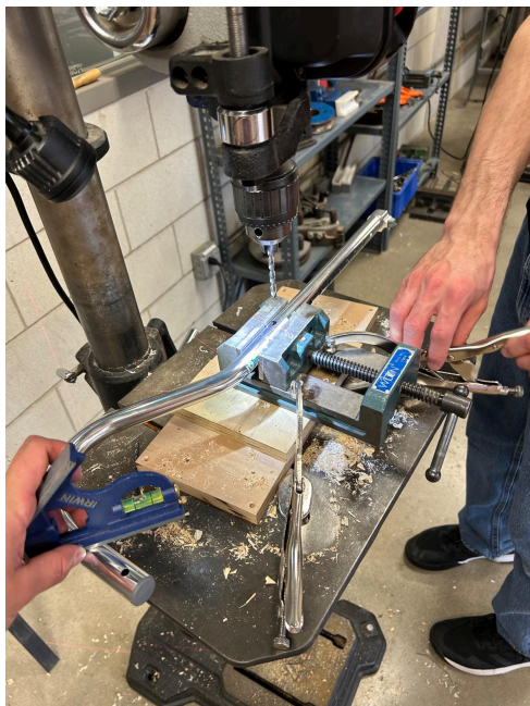
Fig. 9: Drilling first shaft hole
