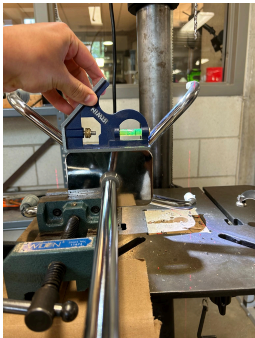
Fig. 3: Cane in vice and aligning under drill press
